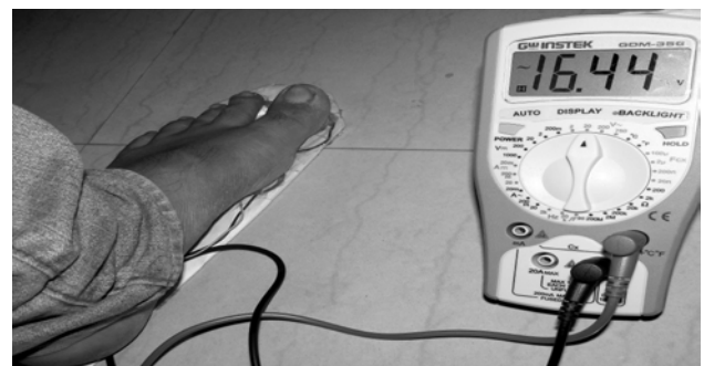
Fig. 4: Snapshot of the project work while voltage generated from Piezoelectric sensors
